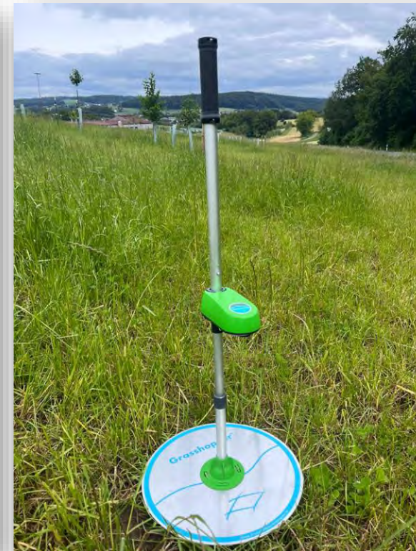
Grasshopper platometer for determination of forage uptake through grazing
